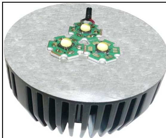
Figure 7: LEDs on Heat Sink Surface
