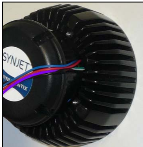
Figure 5: Running SynJet PAR30 LED Cooler Power and Control Wires
